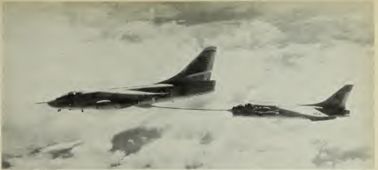
PRECISION air-to-air refueling of jet is made by Navy A3 Skywarrior as it connects its fuel drogue to F8 Crusader.
